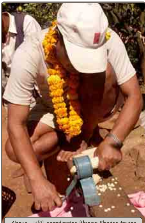
Above - HPG coordinator Bhuvan Khadga trying out a maize de-huller in Purano Gaun. A time trial demonstrated that the simple machine, costing NRs 600/- (about £4.50) was 3 times faster than doing by hand, though this figure will increase as de-hulling by hand gets slower because hands will tire and develop blisters.
