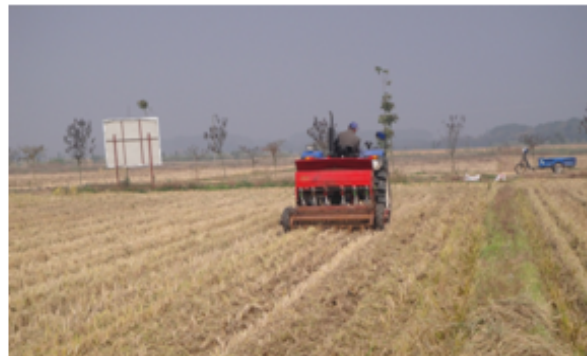
(2) Winter wheat seeding after rice harvesting with straw recycling and little tillage in the fixed furrow
