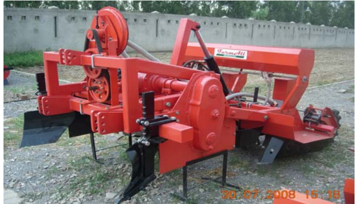
Bed renovator with precision pneumatic seeder and fertilizer applicator
